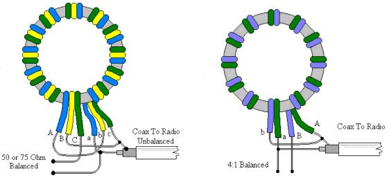
Winding and connection detail.
