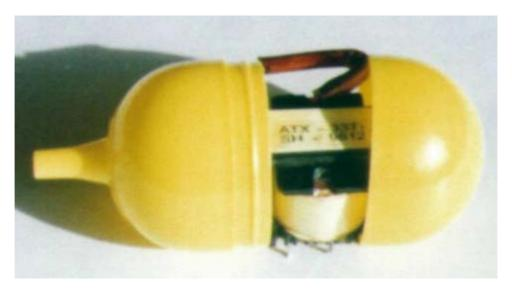
Second variant of the connection for AT- 33T transformer Second variant of the connection of a RF transformer
