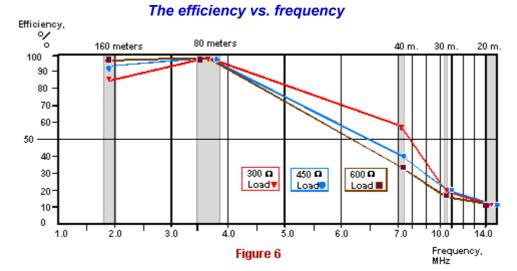
The most important parameter of any RF transformer is its efficiency. This RF transformer (Fig. 3) has a high efficiency only on ranges of 160 and 80 meters. The efficiency falls up to 60-35 percent (it depends on the
